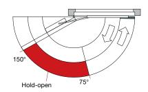
OPENING LIMITER MODULE FOR SLIDE ARM GR400/450/500/3400/3500
