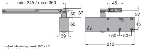
1: adjustable closing speed 180° - 15° 2: adjustable latching 15°- 0° BC: adjustable backcheck 70° - 180°
