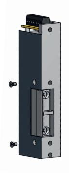
An electrically operated lock-bolt model of 24 V DC, 58 mA, 1.39 Watts, equipped with feedback contacts (locked / unlocked door and closed door) as a standard.
